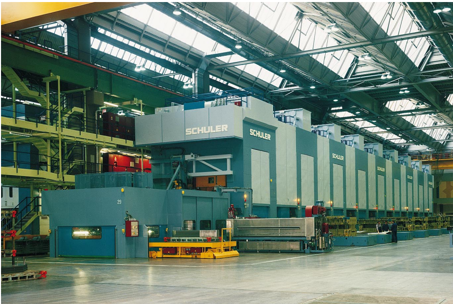
▲ Fig. 4.4.19 Mechanical press line with noise protection (double-action lead press, nominal press force 20,000 kN, follow-on single-action presses, nominal press force 15,000 kN)
