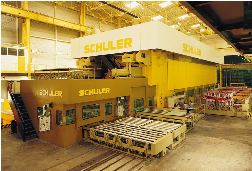
▲ Fig. 4.4.15 Destacker of a large-panel transfer press for maximum blank dimensions of 3,800 \times 1,800 mm with a destacking bridge
