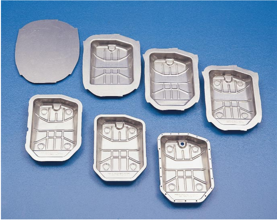
▲ Fig. 4.1.1 Production steps for the manufacture of an oil sump
