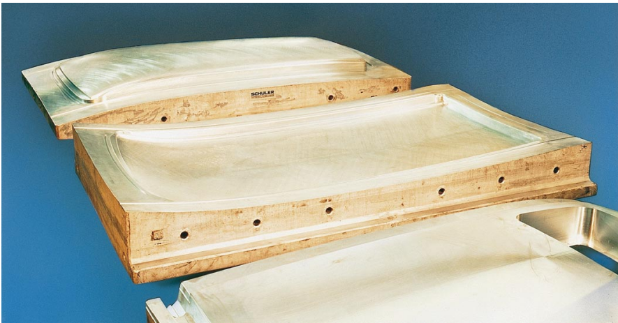
▲ Fig. 4.1.13 Prototype drawing die in aluminium for the production of the roof of a station wagon
