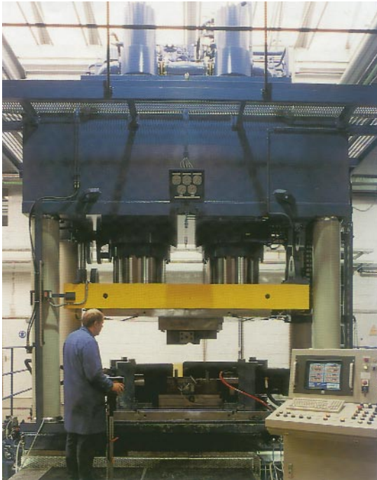
◀ Fig. 5.6.1 Four-upright hydroforming press with a closing force of 25,000 kN
