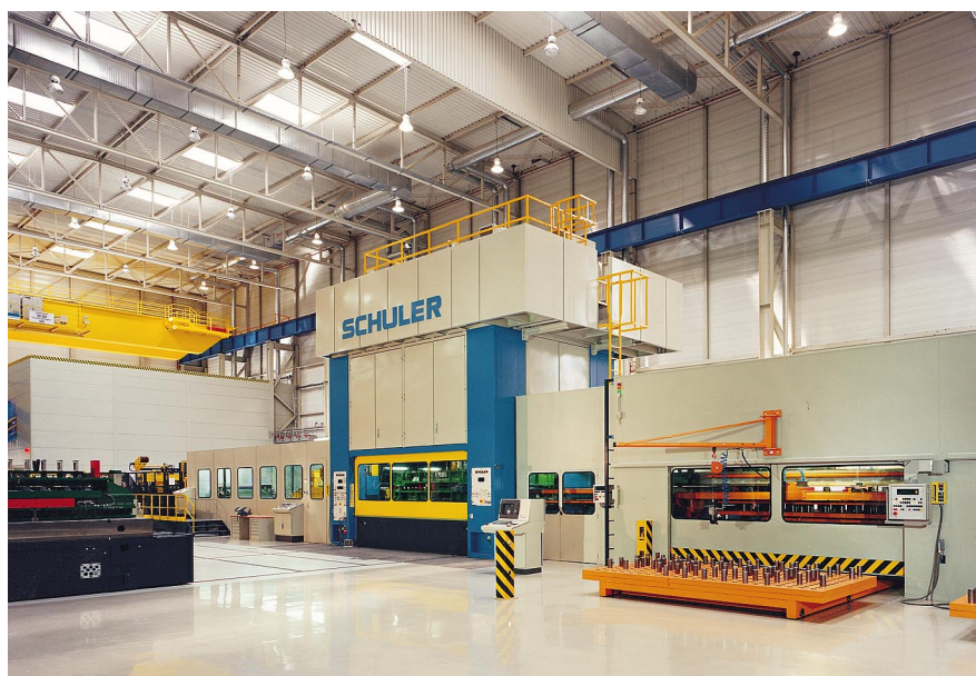
▲ Fig. 4.6.5 Contour blanking line with nominal press force of 8,000 kN (six-link drive)
