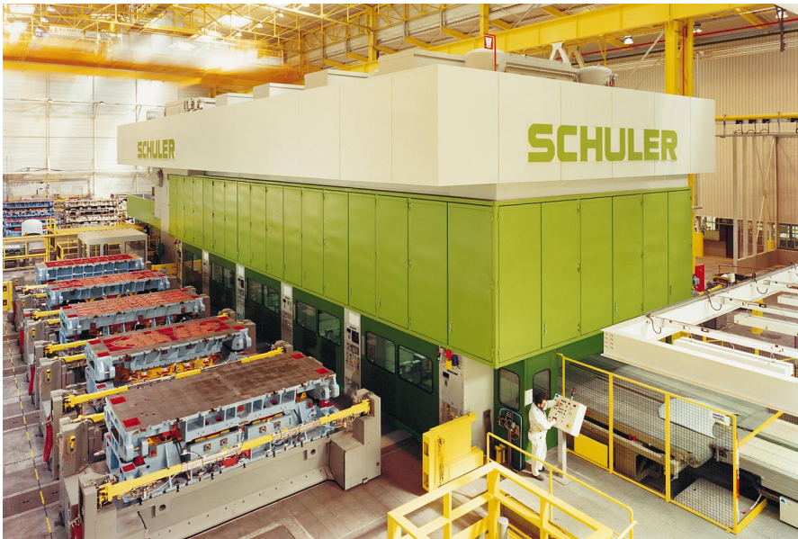
▲ Fig. 4.4.38 Crossbar transfer press with moving bolsters outside the press nominal press force: 52,000 kN; slides: 5; work stages: 5; feed pitch: 2,000 mm
