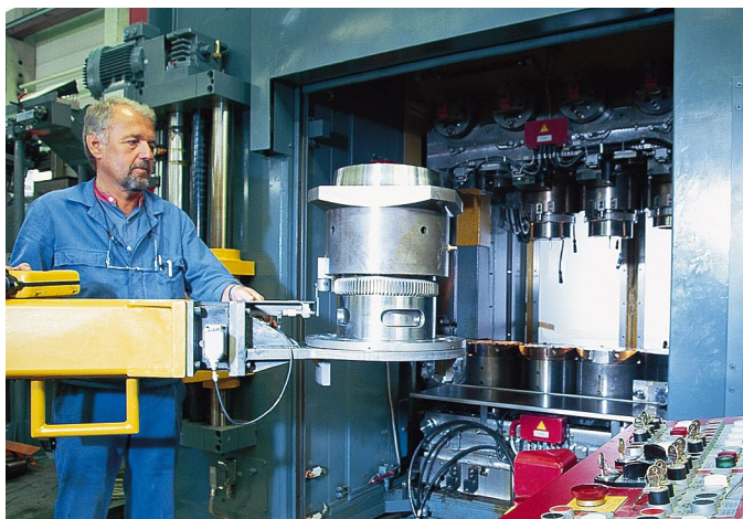
▲ Fig. 3.4.5 Die changing arm for solid forming
