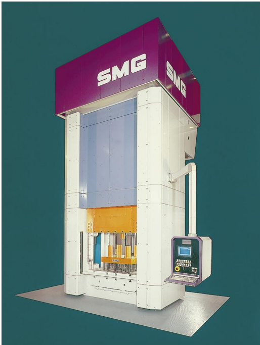
◀ Fig. 4.4.1 Hydraulic universal press (nominal press force 5,000 kN)
