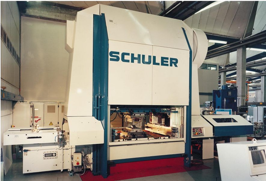
▲ Fig. 4.4.5 Hybrid press (nominal press force 3,150 kN)
