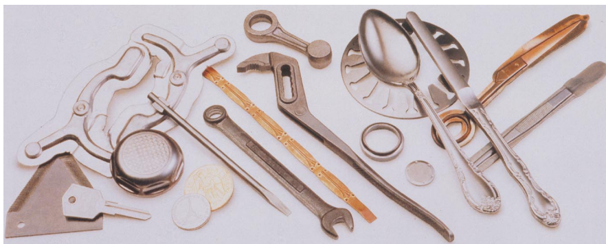
▲ Fig. 6.1.4 Examples of coined parts, such as coins, medals, cutlery and various hand tools, as well as cold-coined hot forged parts
