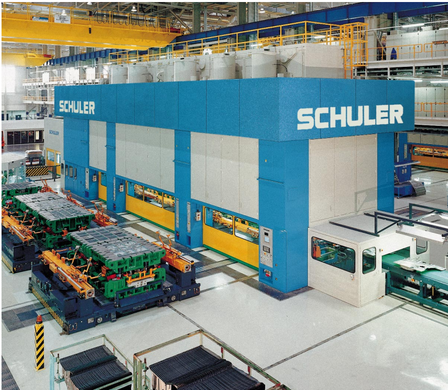
▲ Fig. 4.4.27 Large-panel tri-axis transfer press nominal press force: 38,000 kN; slides: 3; work stations: 6; feed pitch: 2,000 mm; strokes per minute: 8-18
