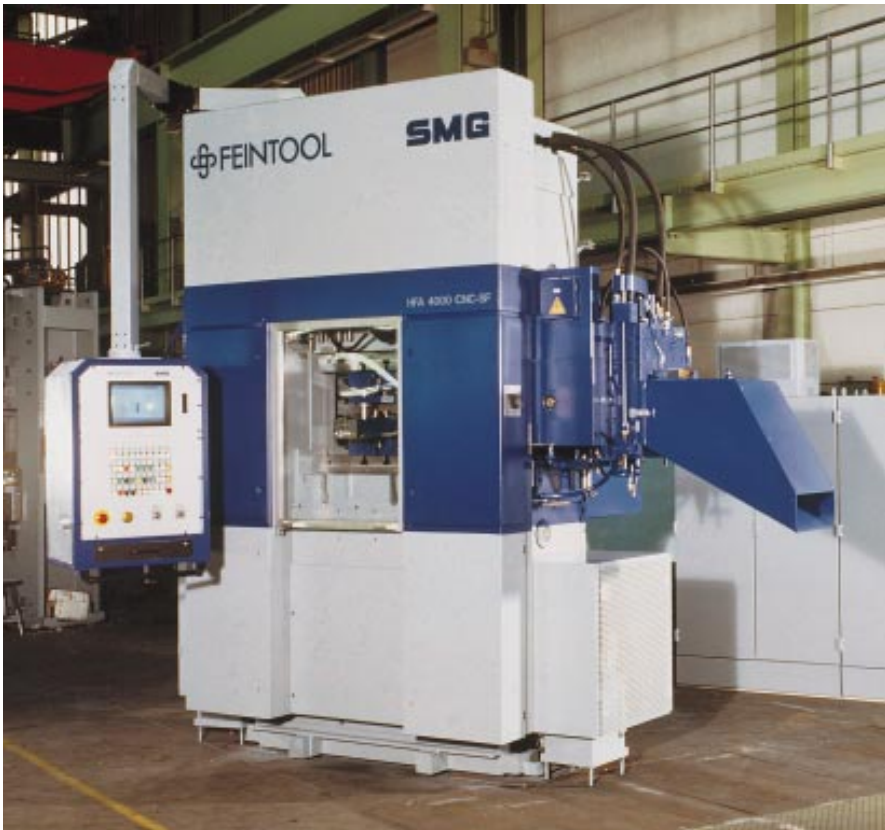
▲ Fig. 4.7.30 Fine blanking press with a nominal press force of 4,000 kN
