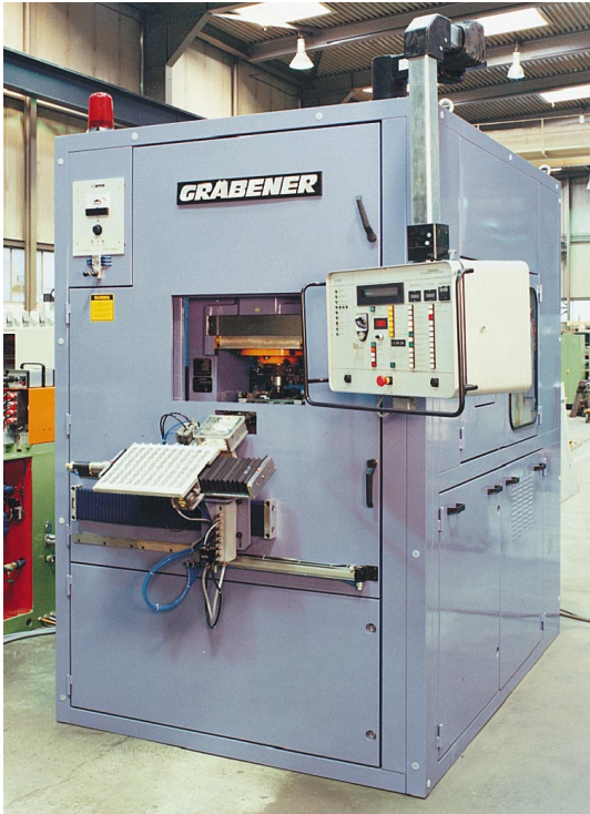
◀ Fig. 6.8.27 Medal minting press with manual feed
