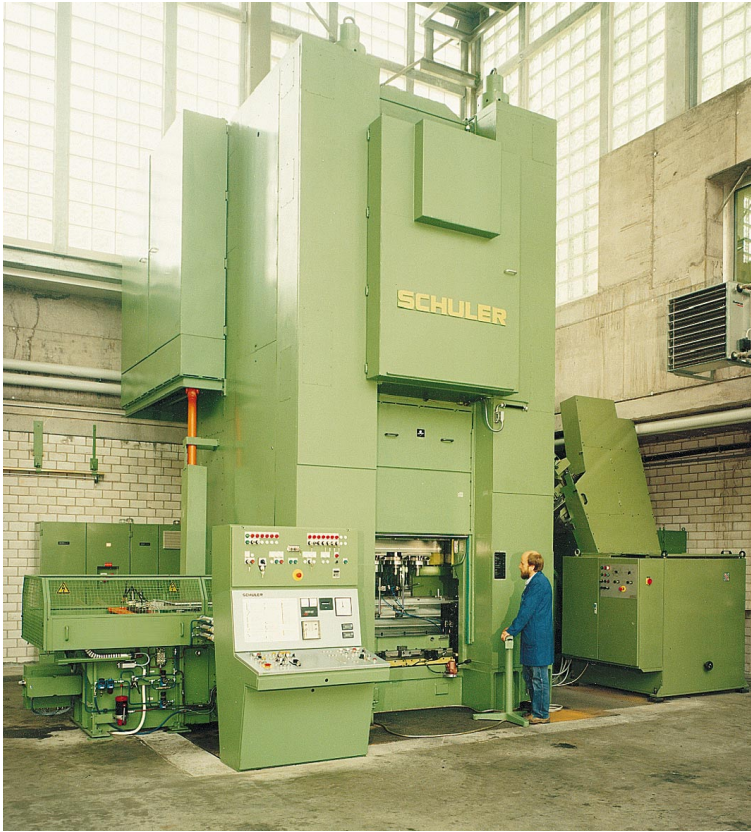
▲ Fig. 6.8.4 Multiple-station press with modified knuckle-joint top drive (nominal press force 10,000 kN, four stations, loading system and transfer feed)
