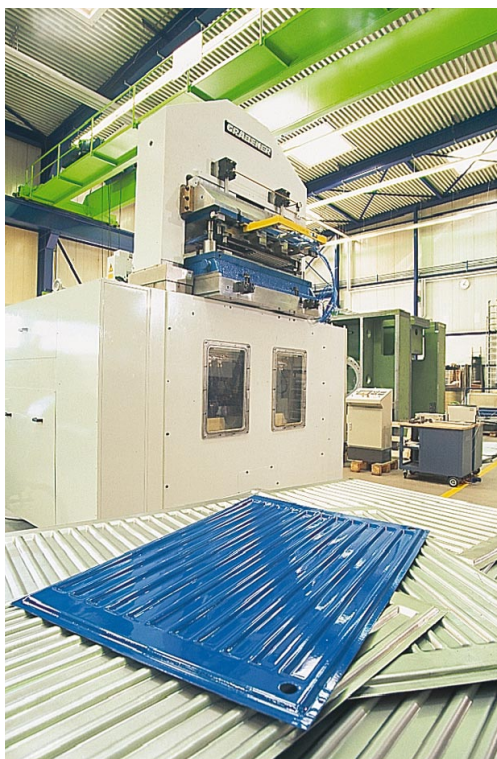
◀ Fig. 4.4.11 Bottom drive knuckle-joint press for the manufacture of flat radiator plates (nominal press force 6,300 kN)
