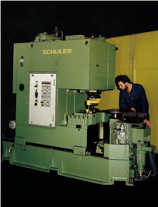
◀ Fig. 4.6.14 Notching machine for circular blanks with numerical indexing drive system (nominal press force 250 kN)
